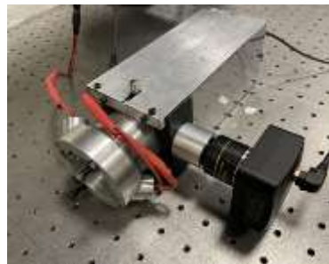
Indigenously developed VIS – NIR Spectrometer
