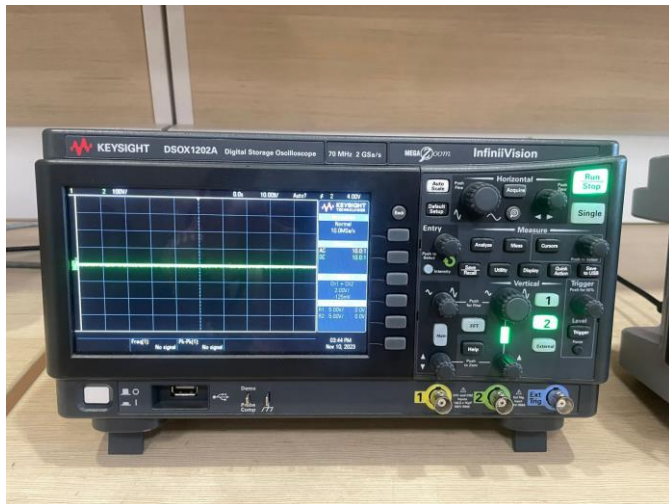
Digital Storage Oscilloscope DSOX1202A/ 70Mhz, 2GSa/s Make- Keysight Technologies
