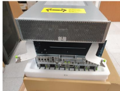
The rear of the DGX A100 with the upper GPU tray removed and placed on top.
